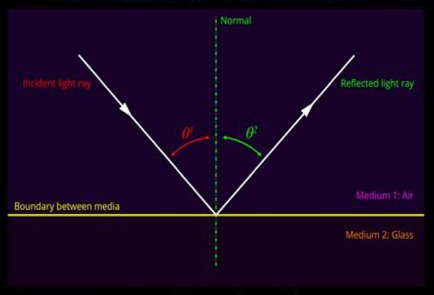
When a ray of light reflects off a smooth surface the angle of incidence (θ') is equal to the angle of reflection (θ').
