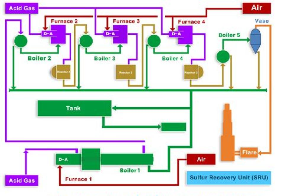
Figure 1. Sulfur recovery unit (SRU) process flow diagram.
