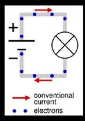
Note current moves from positive to negative, however electrons are actually are moving in the opposite direction!
