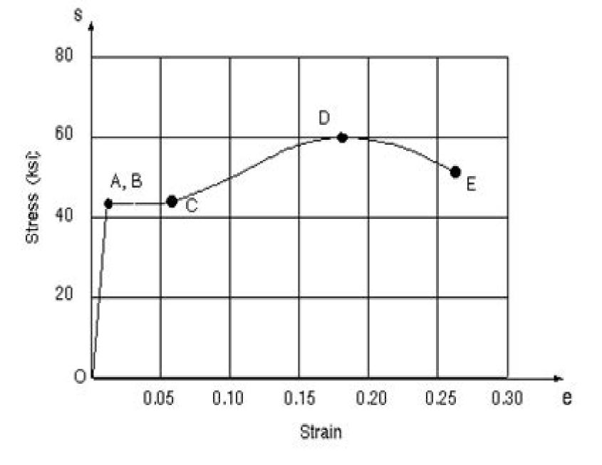
Figure 3. Stress-strain diagram for structural steel in tension.
