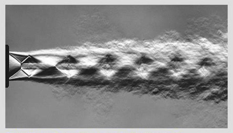
The complex interactions between shock waves and expansion waves in an "overexpanded" supersonic jet. The flow is visualized by a schlierenlike differential interferogram.
