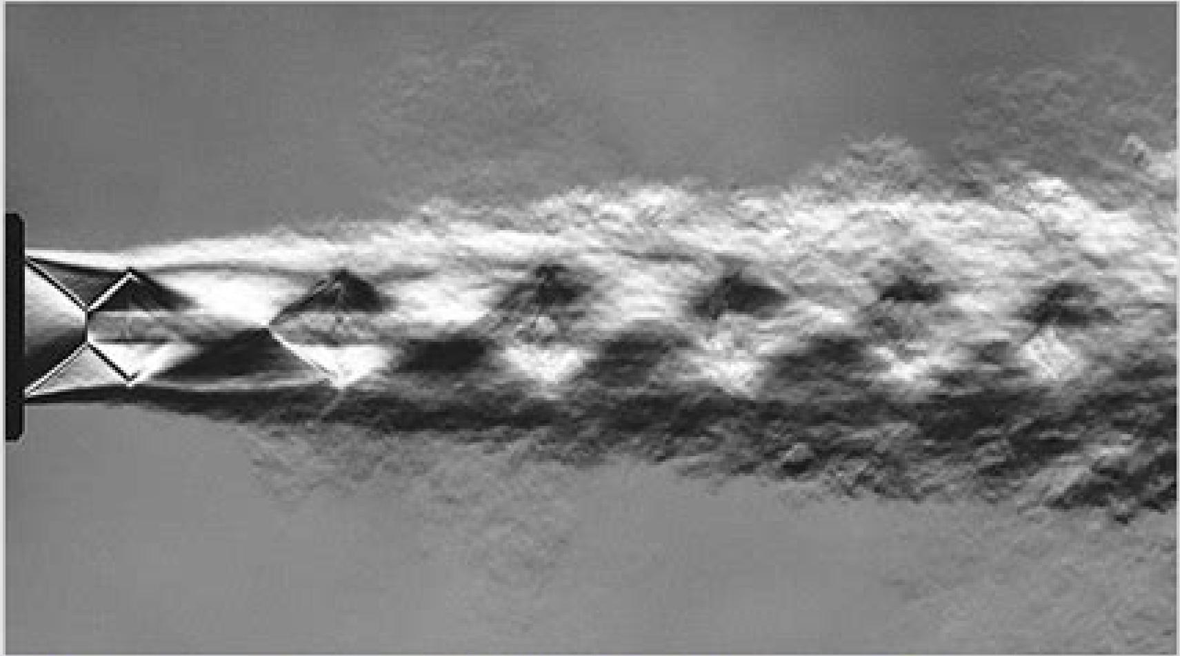
The complex interactions between shock waves and expansion waves in an "overexpanded" supersonic jet. The flow is visualized by a schlierenlike differential interferogram.
