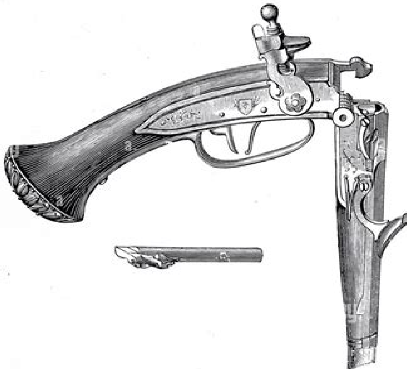
Early Breech-loading Flint-lock Pistol.
