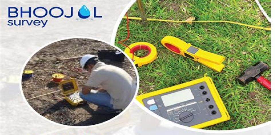
Soil resistivity test determine low resistivity zone for design of grounding system, Earthing systems. On the basis of field data collected and earthing test report generated type of grounding design system i.e Electrode earthing, Chemical Earthing can be determine.
