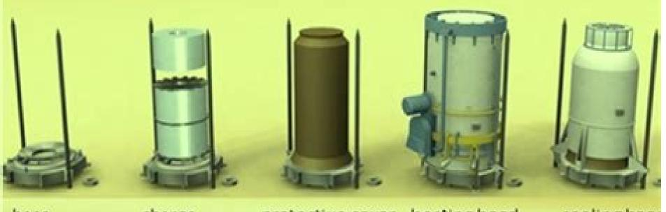
base charge protective cover heating hood cooling hood
