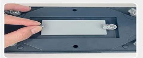
Remove and unlock the battery cover
