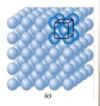
Fig.4.2: BCC Crystal Structure
