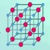
Particles are close-packed so they can vibrate, but not flow.
