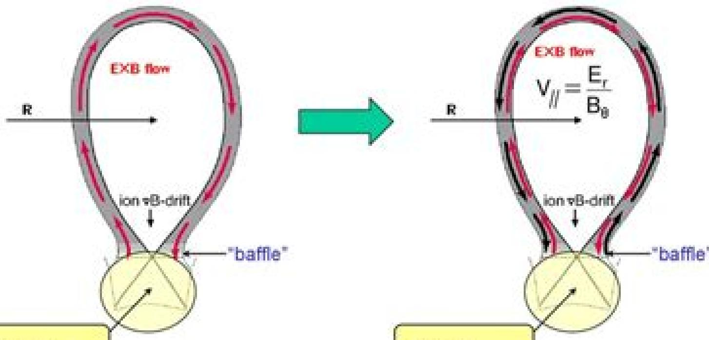
Poloidal ExB Drift + Parallel Flow = Toroidal Flow
