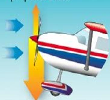
Load on downward moving propeller blade
