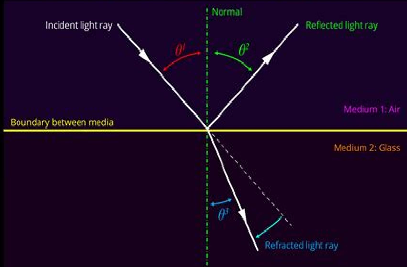
Angle of incidence  $\theta^i$  = Angle of reflection  $\theta^r$ . Angle of refraction  $\theta^t$ .
