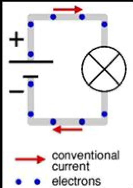
Note current moves from positive to negative, however electrons are actually moving in the opposite direction!
