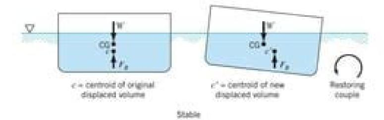
Note: Center of gravity of the volume (centroid) of fluid displaced is also the center of buoyancy.
