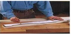
Make a sturdy template from hardboard or another durable material when making multiple parts with the same profile.
