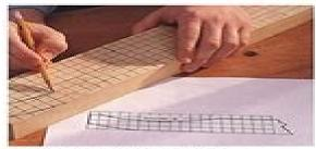
Transfer grid drawings to your workpiece by drawing a scaled grid, then recreating the pattern using the grid as a reference.
