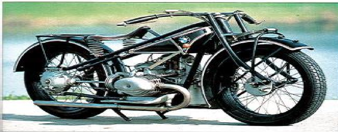
The R47 of 1927 replaced the R37, having an improved 494cc engine.
