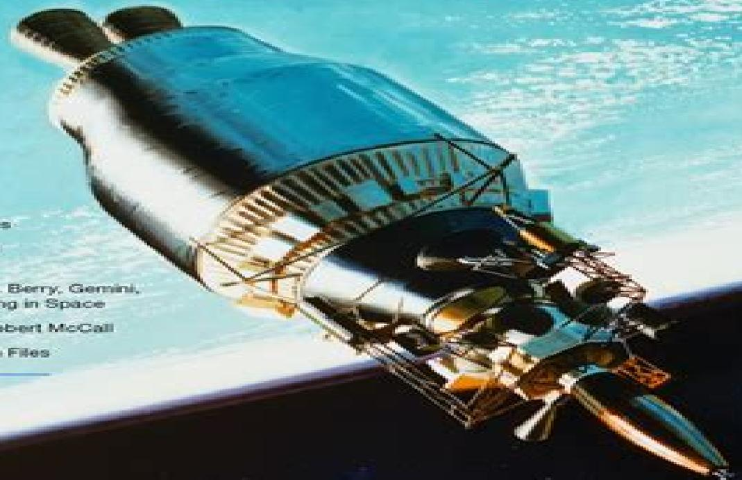
21 An illustration depicts the Galileo spacecraft being deployed with Shuttle-Centaur. (Credit: NASA)
