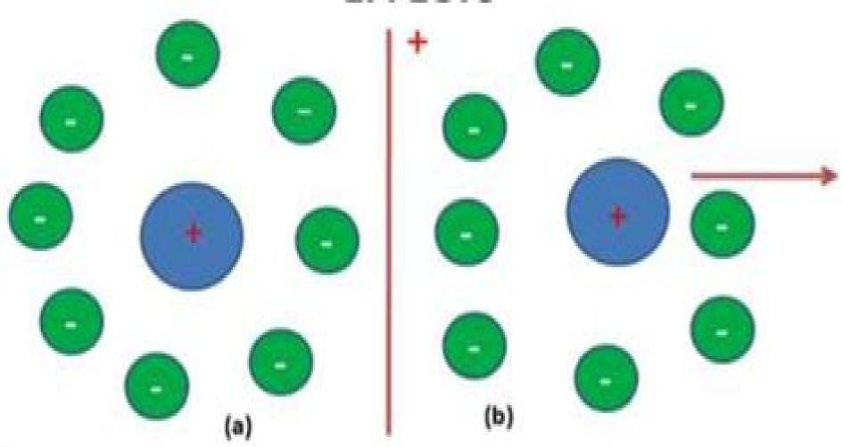
Symmetrical ionic atmosphere around a positive ion Ionic atmosphere becoming asymmetrical when central ion moves
