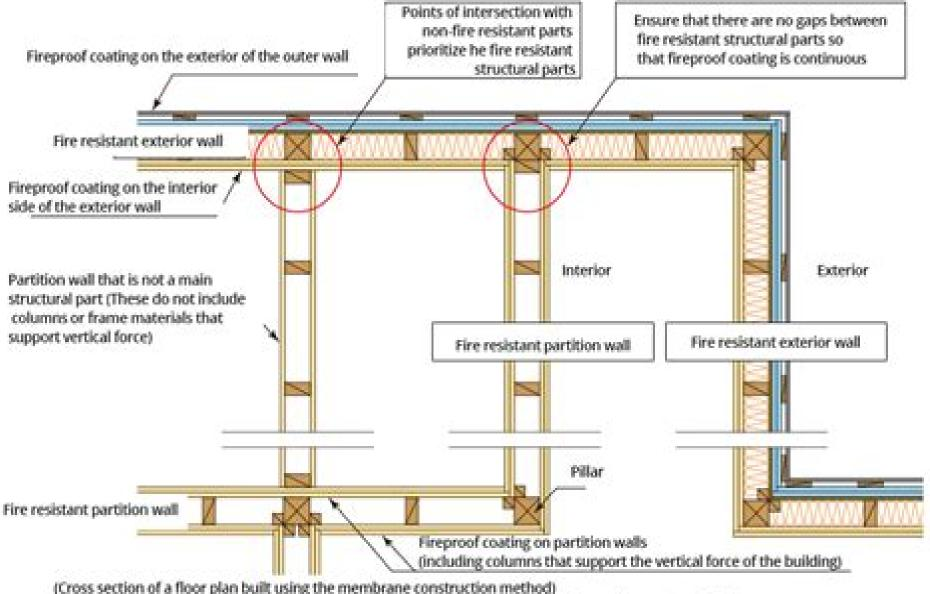
(Cross section of a floor plan built using the membrane construction method)
