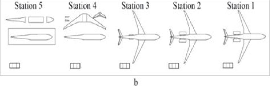
Fig. 1. (a) Bench layout (b) Flow line layout
