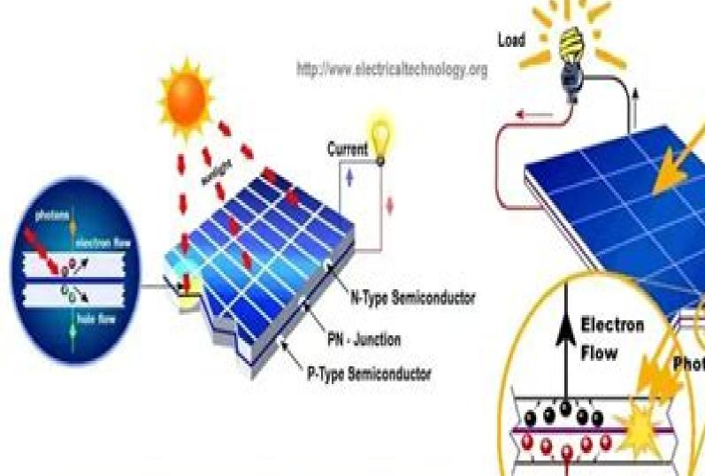
Basic Operating Principle of a Solar Cell
