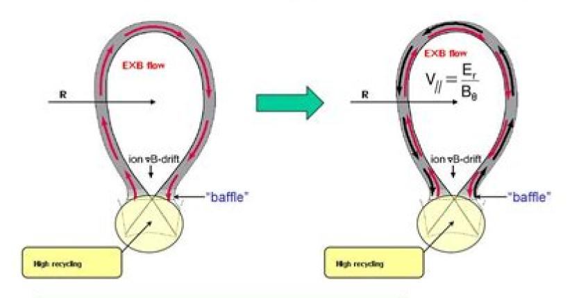
Poloidal ExB Drift + Parallel Flow = Toroidal Flow
