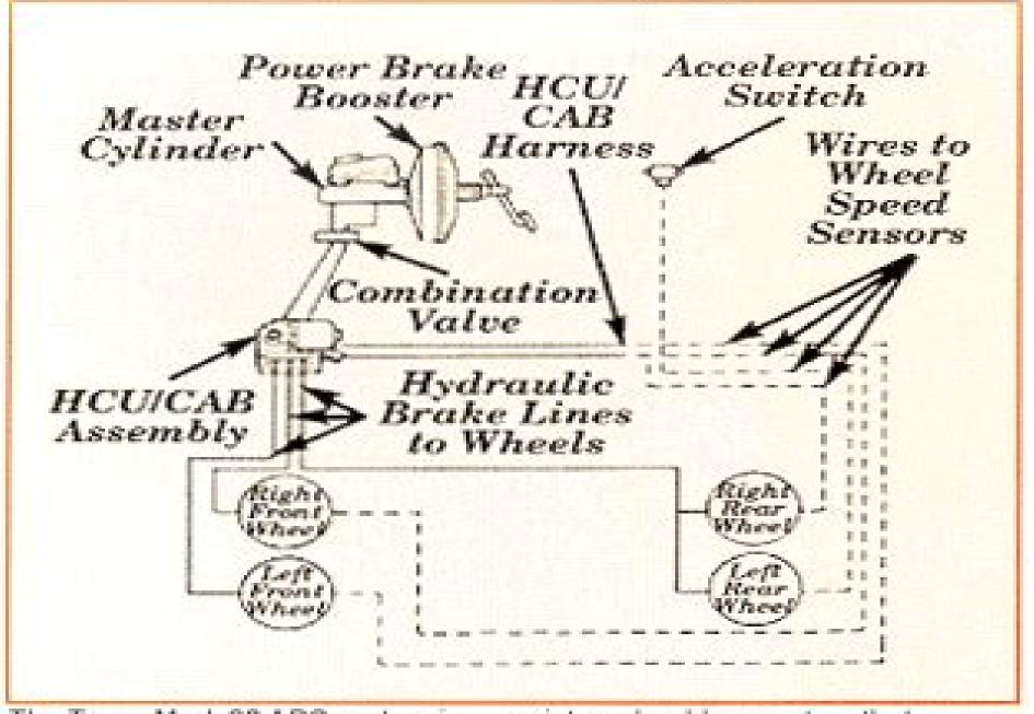
The Teves Mark 20 ABS system is a nonintegral, add-on system that uses a conventional vacuum booster and master cylinder (illustrations courtesy DaimlerChrysler Corp.).
