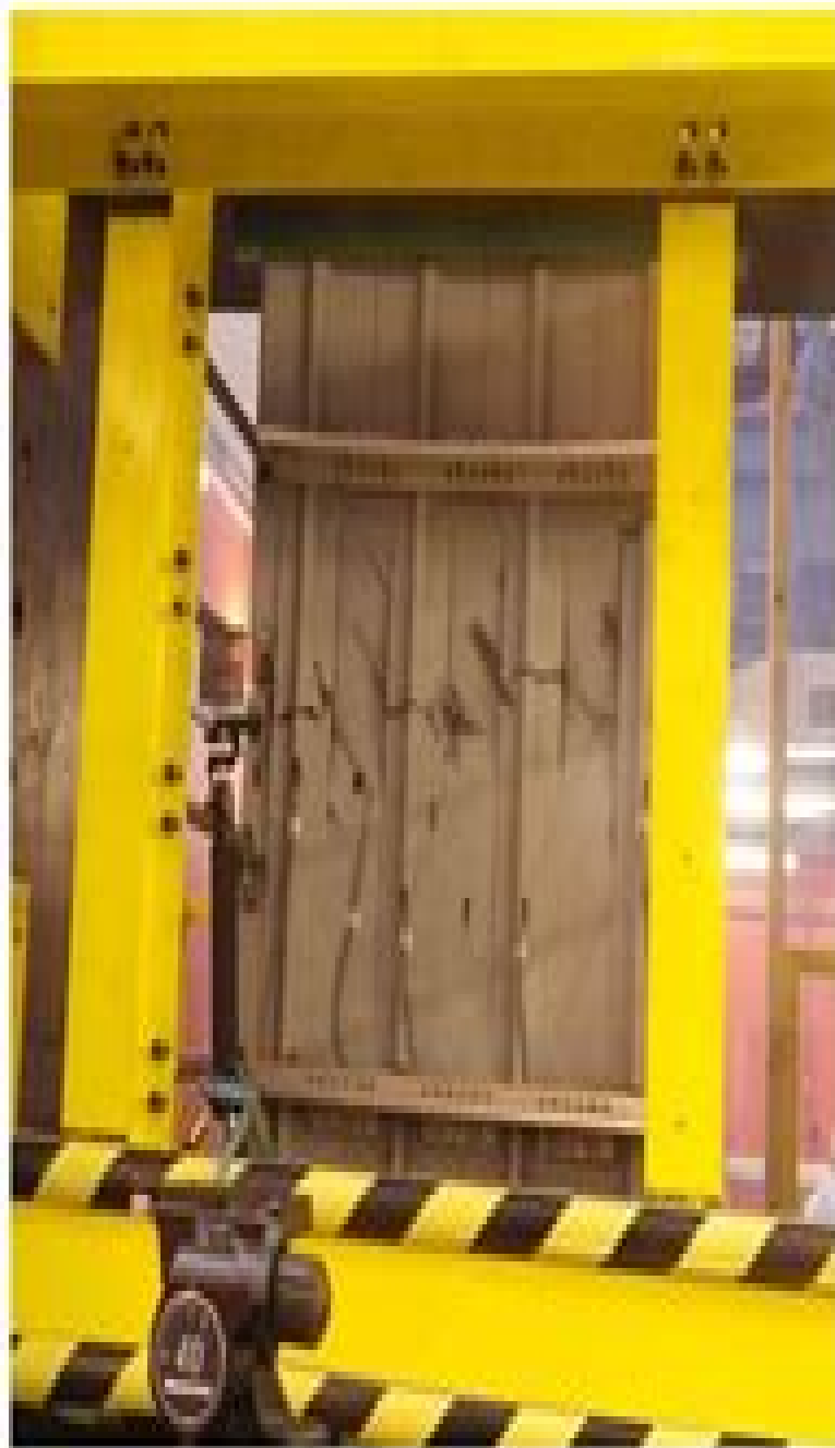
Fibre Compressive Damage
