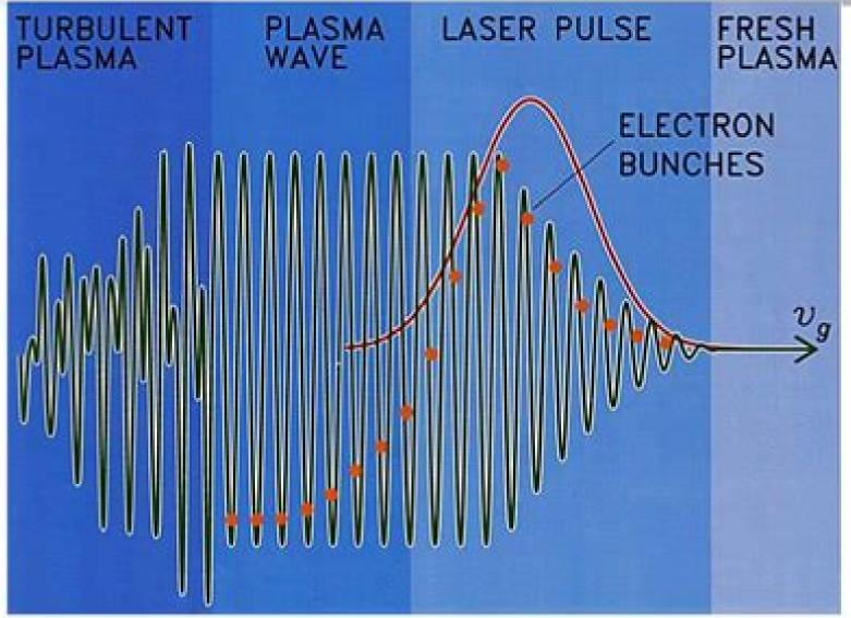
Ion dynamics becomes important: strong plasma turbulence driven by electron plasma waves destroys the accelerating wave structure.
