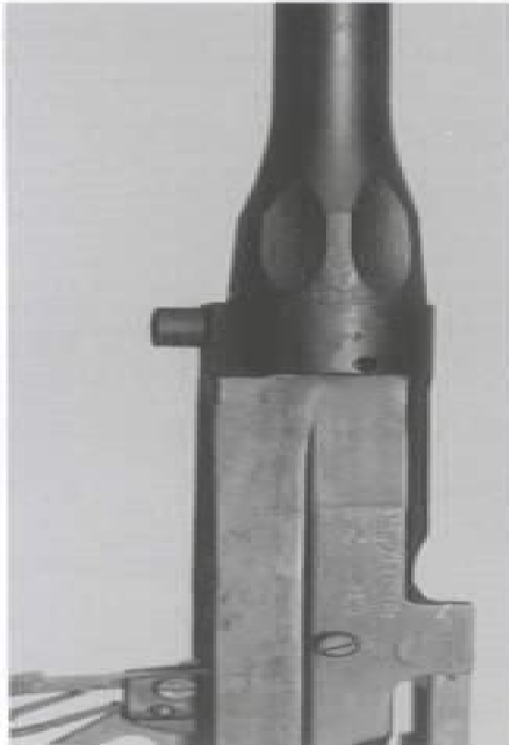
These two views of the Number 5 rifle show some of the lightening cuts which were made in order to shave weight from the rifle. At left, the dished out cuts in the barrel's chamber area are quite evident, while at right, metal at the bottom of the receiver was judiciously removed.
